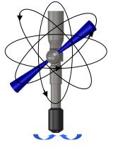
The rotary movement of the spray head around all axes forms a 360° spray pattern, which means that every point in the container is sprayed with cleaning agent.
